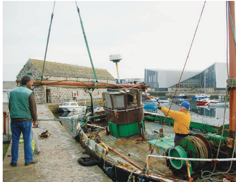
The first mast is removed from the boat
